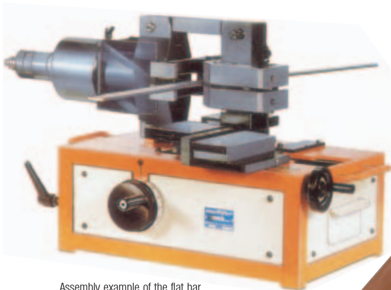
Assembly example of the flat bar bender tool art. 9153
