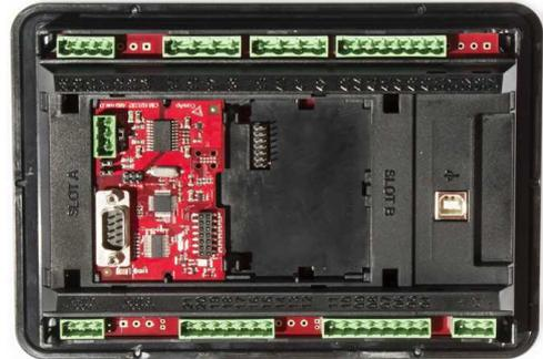
After locking the plug-in module into holders, place back the back cover (small cover for connectors has to be removed from back cover). Finally insert the small cover for connectors. Small covers are unique for each plug-in module.
