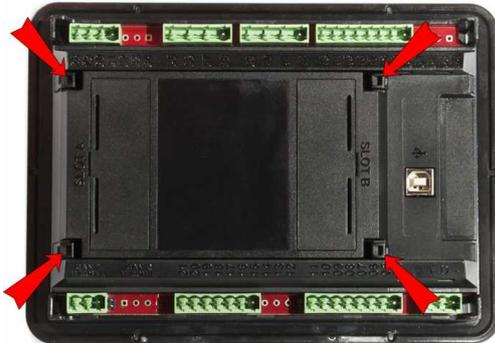
After removing back cover insert the plug-in module. Plug-in module has to be inserted under holders. Start with holders marked by symbol 1. On the controller are also narrow for better navigation. After inserting plug-in module under holders 1 press it down to holders marked by symbol 2 which lock the module.
