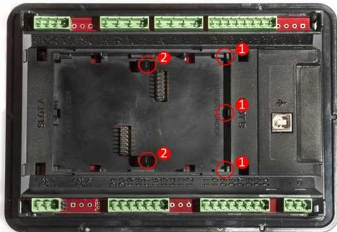
Insert the plug-in module under holders marked by symbol 1. Then insert the plug-in module under holders marked by symbol 2.
