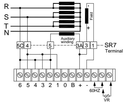
Figure 15 1 phase 220 Vac With auxiliary winding
