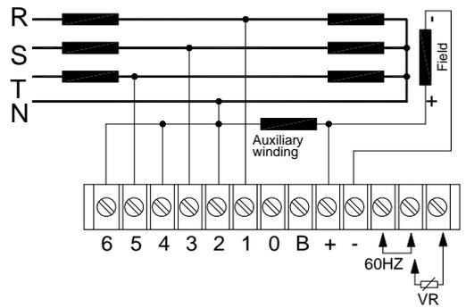
Figure 13 3 phase > 480 Vac With auxiliary winding
