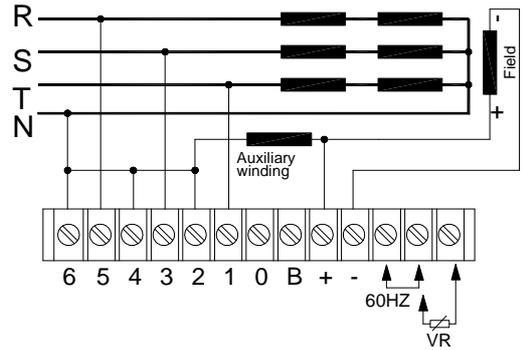
Figure 11 3 phase 380 / 480 Vac With auxiliary winding
