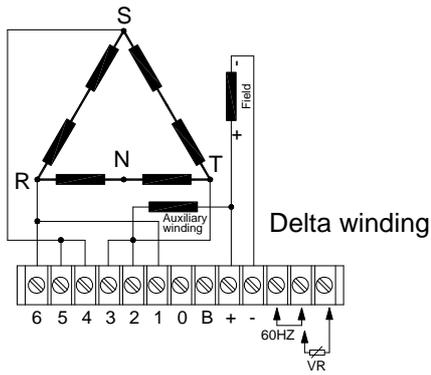
Figure 3 3 phase 240 Vac With auxiliary winding
