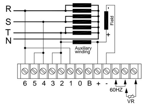
Figure 9 3 phase 220 Vac With auxiliary winding
