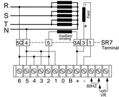
Figure 17 1 phase 380 / 480 Vac With auxiliary winding
