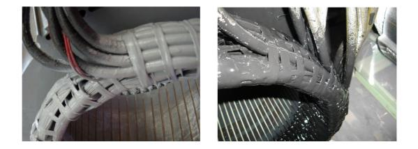
Grey treatment (marinization) on the left, TOTAL+ treatment shown on the right. The EG43 grey varnish, is an high temperature insulating enamel that forms a tough and flexible film, with excellent moisture and chemical protection. It is water and oil proof, and also protects windings from abrasion. It is applied spraying an over coating layer over the impregnated winding, or dipping the stator in a varnish barrel for superior treatments
