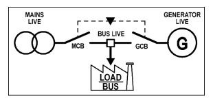
measures to determine when the **Mains** is back. When the **Mains** is back, the device command the **MCB** and **GCB** circuit breakers to supply the **Loads** by the **Mains**.
