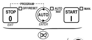
PROGRAM (Engine Stopped) By means of the STOP and AUTO buttons pressed together, it is possible to enter the configuration menu and adjust the available parameters (some parameters may require a password).
