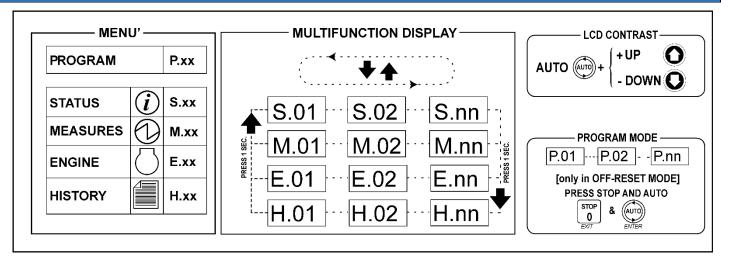
This area, which is composed by a display and the buttons, allows the visualization of the configuration parameters, the plant status, the electrical measures, the engine analogue and digital measures, the digital IN/OUT signals acquired and the historic visualization of the events and the measures.
